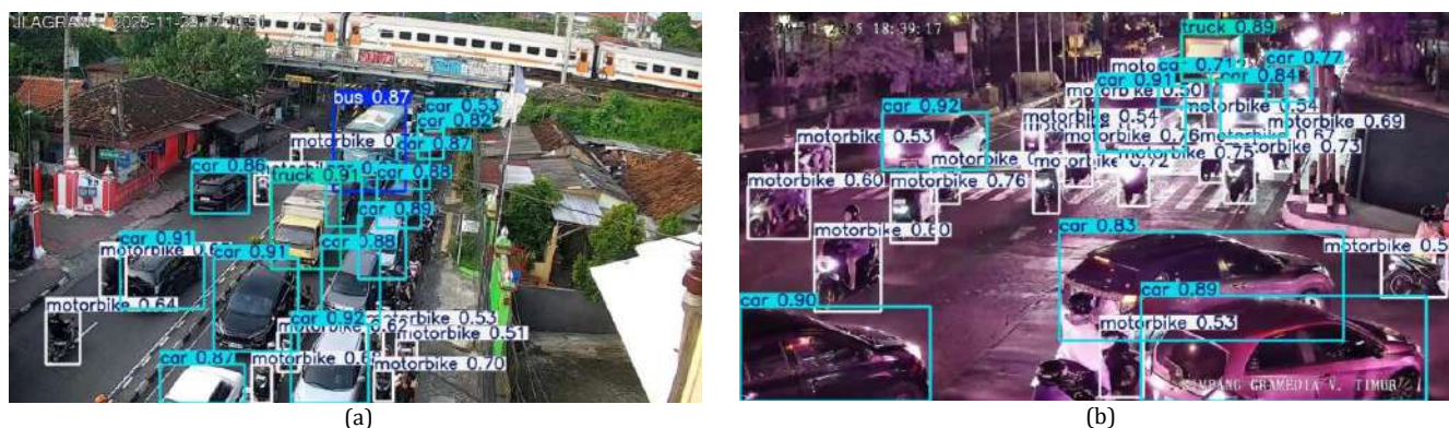
Fig. 7. Vehicle detection results using the Domain Adaptation model under (a) daytime and (b) nighttime conditions.
