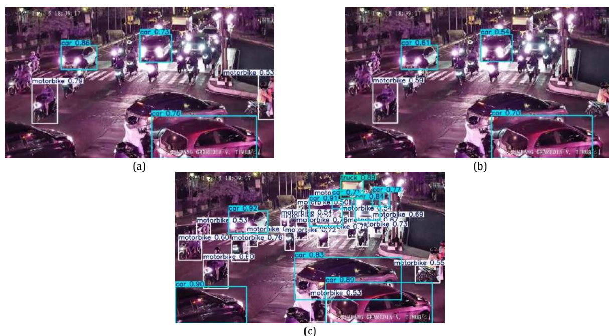
Fig. 12. Comparison of vehicle detection results under nighttime conditions using the (a) Base Training, (b) Fine-Tuning, and (c) Domain Adaptation models.
